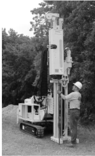
The Geoprobe® Automatic Drop Hammer mounts on any Geoprobe® 66DT or 6610DT. The drop hammer is not dedicated to one machine. Remove one pin and attach the overhead winch to begin unmounting. The drop hammer can be stored upright and out of the way.
