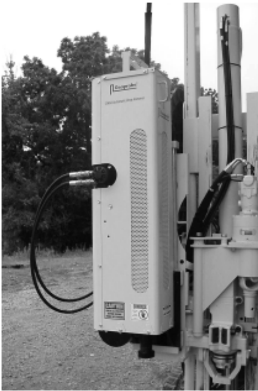
The Geoprobe® Automatic Drop Hammer is equipped with a 140-pound hammer with a 30-inch chain-driven drop.
